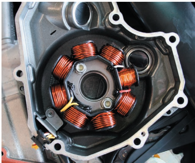
2-A. Install Trail Tech stator.
